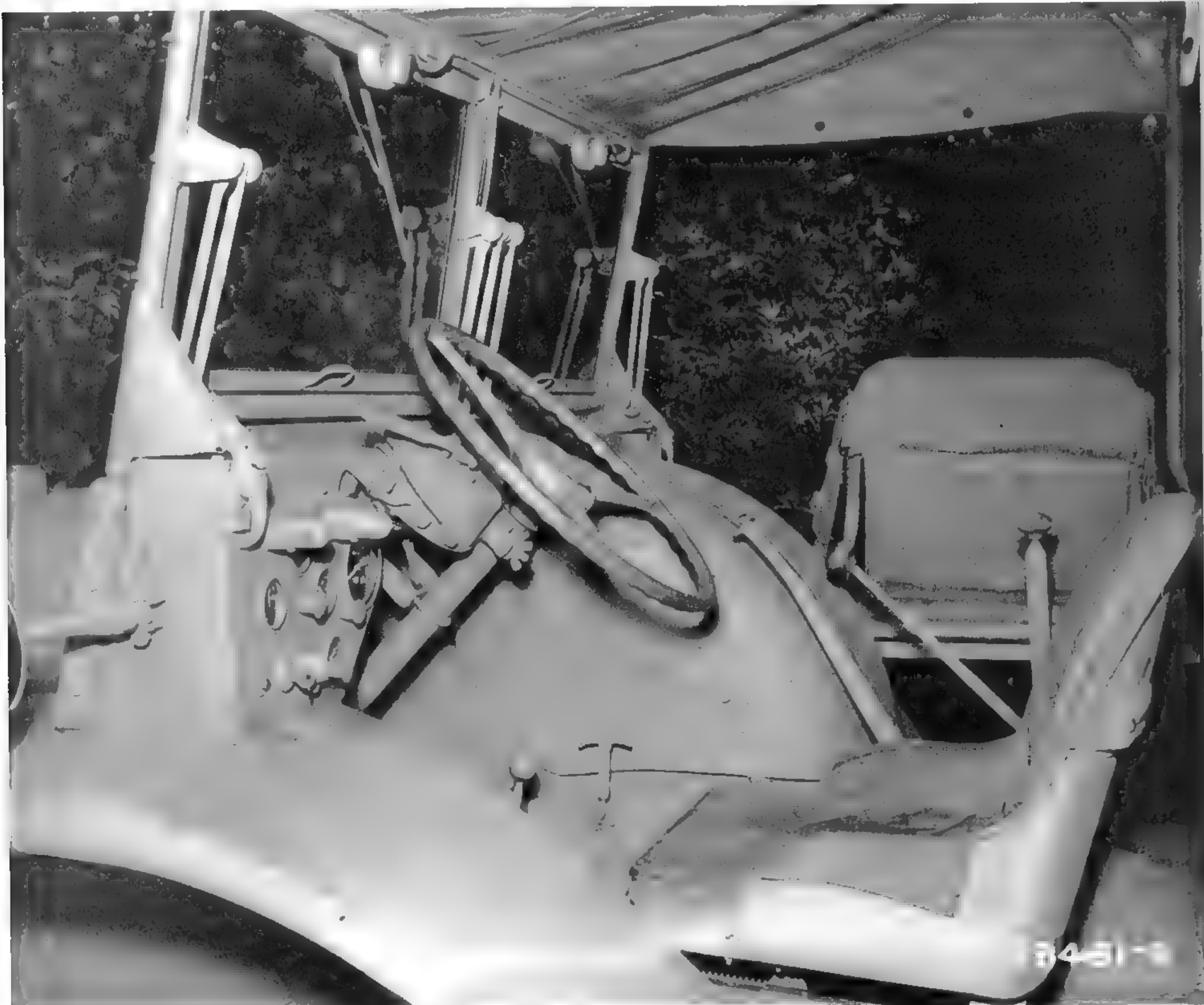
This is the interior of a GTBC. The cab layout of all the vehicles in the GTB-family was very similar. Notice the sideways-facing passenger's seat. The GTBC was equipped with an electric brake controller, which can be seen mounted on the steering column, just above the instrument panel. (Photo courtesy of the Bryce Sunderlin collection)
